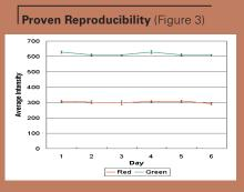
The GenePix 4000B Scanner offers proven repeatability, scan after scan. A non-bleaching fluorescent test standard was scanned repeatedly and the average signal was quantified. Signal value variance among all scans was 1.6% in the green channel and 2.1% in the red channel. Error bars cover two SD from the mean of the four measurements at each time point.
